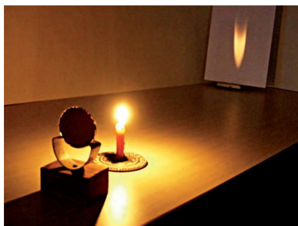
Fig. 15.15 Real images formed by a concave mirror
