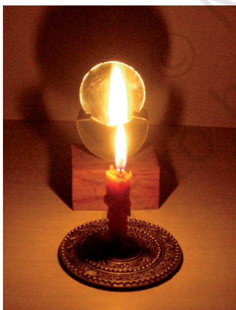
Fig. 15.16 Virtual image formed by a concave mirror
