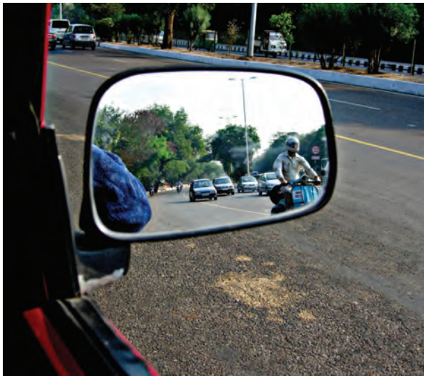
Fig. 15.20 Convex mirror as side view mirror
