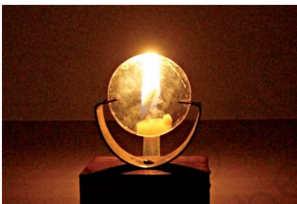
Fig. 15.26 Virtual image formed by the convex lens
