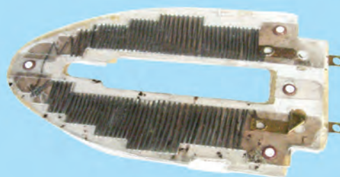
Fig. 14.11 Element of electric iron
