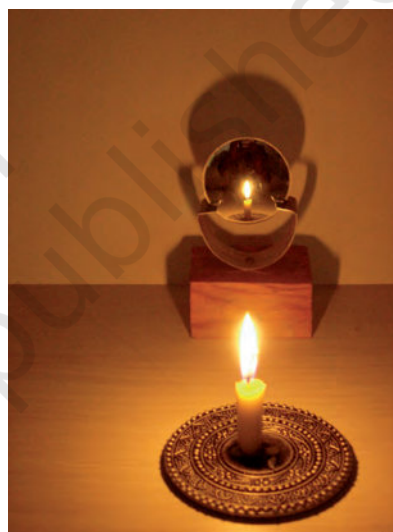
Fig. 15.19 Image formed by a convex mirror
